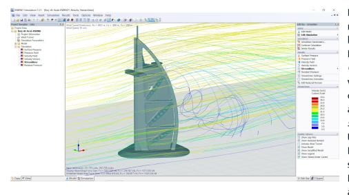
Simulation **RWIND** numerical model is based OΠ Finite-Volume code OpenFOAM. The final volume mesh is created via application snappyHexMesh. The turbulence model is RANS k-ε. A typical simulation time with RWIND Simulation is a few minutes. The
