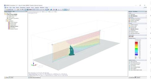
**RWIND Simulation user** interface is super ease of use with minimal necessary settings and skills. The user workflow is very simple. The input for RWIND Simulation is the surface model of the structure (CAD, .STL). The virtual wind tunnel is created around the structure. Wind speed is set. The rest of the
