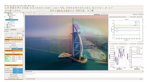
created snappyHexMesh. The tunnel virtual 3000m long, 1000m wide, and 700m high. The mesh is well refined close to the model, including the inflation layers, to model the flow boundary layer as accurate as possible. That leads to the finite volume mesh of about 5,000,000
